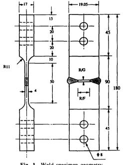
Fig. 1 Weld specimen geometry
