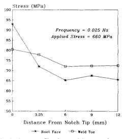
Fig. 2 Stress profiles for partial penetration weld near tip of LOP section and weld toe
